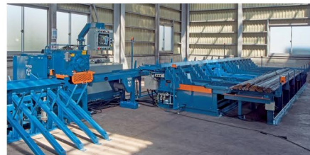
Sorting and feeding device for cutting machine
